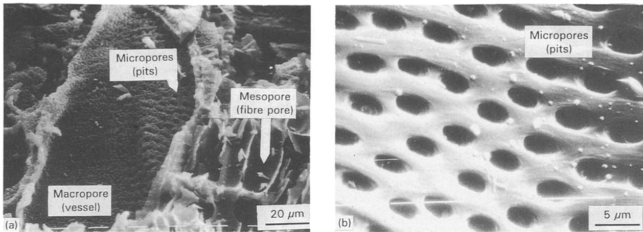
Figure 6 SEM photographs of acacia wood char prepared at 600°C under rapid carbonization. Soaking time = 1 h.
