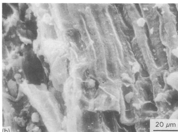
Figure 11 SEM photographs of eucalyptus wood chars prepared at 800 °C under (a) rapid carbonization; (b) slow carbonization. Soaking time = 1 h.
