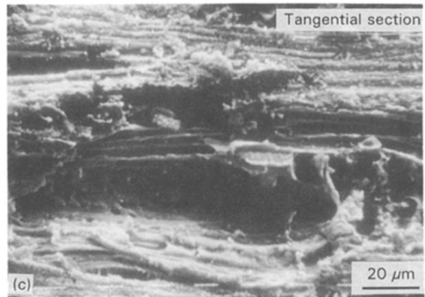
Figure 5 SEM photographs of eucalyptus wood char prepared at 1050 °C under rapid carbonization. Soaking time = 1 h.
