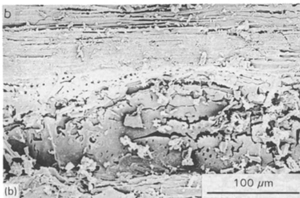
Figure 14 SEM photographs of 1000 °C eucalyptus wood chars prepared after slow carbonization for varying soaking periods (h) (a) 1; (b) 3; (c) 5.
