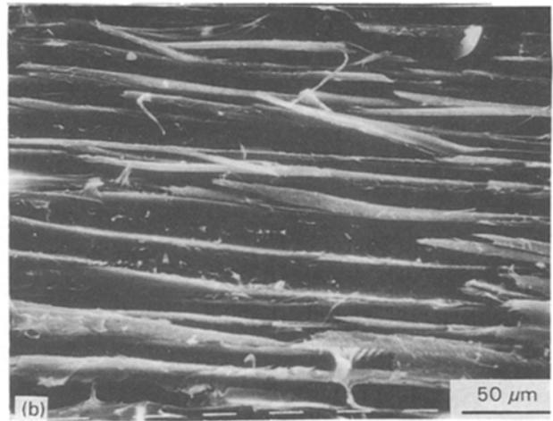
Figure 4 SEM photographs of eucalyptus wood when viewed along (a) radial section (b) tangential section.
