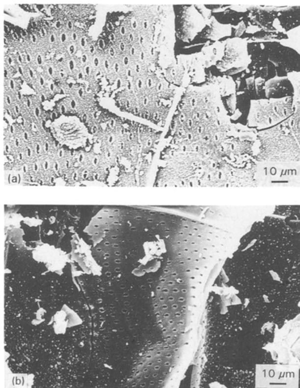
Figure 8 SEM photographs of acacia wood chars prepared under slow carbonization at temperatures (°C) (a) 1000; (b) 1200. Soaking time = 1 h.
