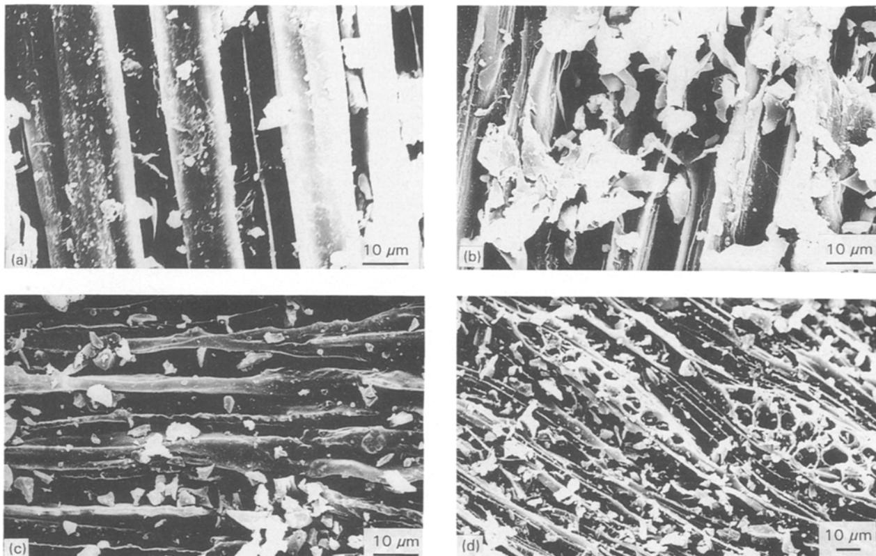
Figure 7 SEM photographs of acacia wood chars prepared under slow carbonization at temperatures (°C) (a) 260; (b) 400; (c) 600; (d) 1000; (e) 1200. Soaking time = 1 h.
