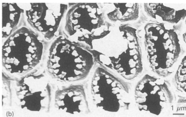
Figure 12 SEM photographs of acacia wood char prepared under slow carbonization at 1000 °C. Soaking time = 1 h.
