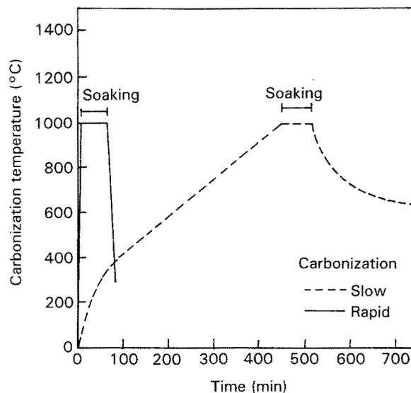
Figure 2 Typical time-temperature profile for slow and rapid carbonization.
