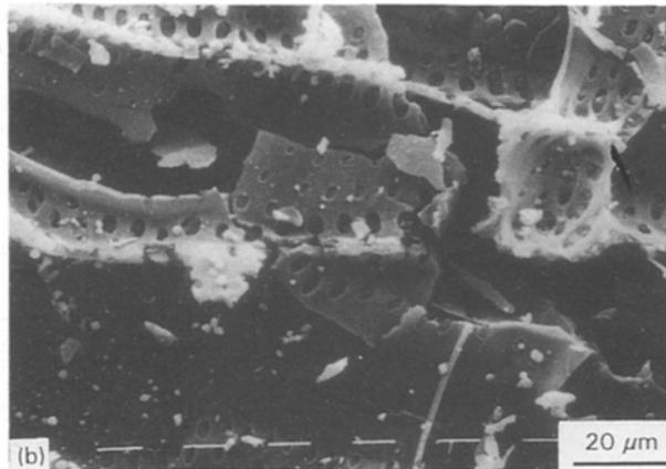
Figure 10 SEM photographs of acacia wood chars prepared under rapid carbonization at temperatures (°C) (a) 800; (b) 1050. Soaking time = 1 h.
