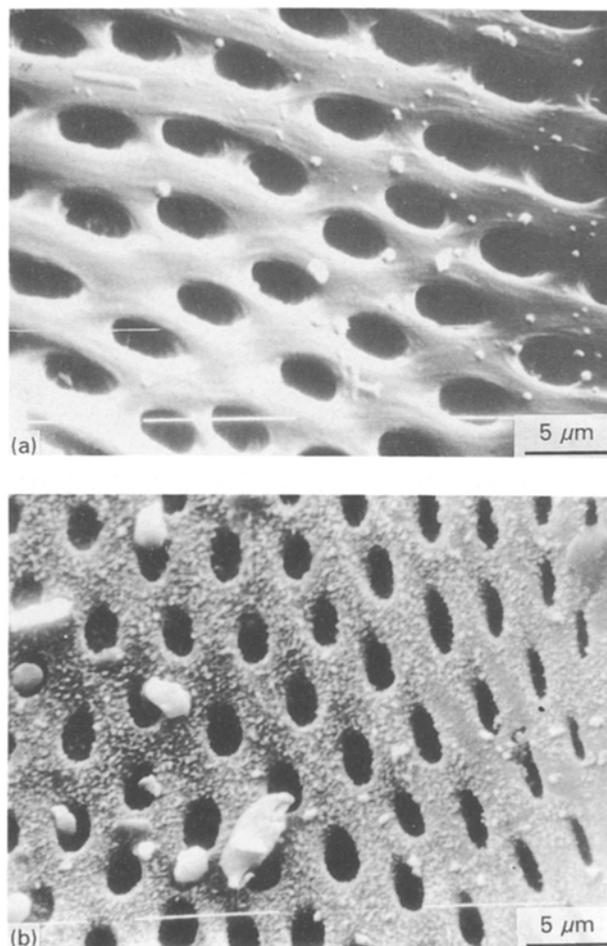
Figure 9 SEM photographs of acacia wood chars prepared under rapid carbonization at temperatures (°C) (a) 600; (b) 1050. Soaking time = 1 h.
